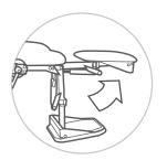
**Fold up footrests**: Hydraulic piston helps switch from footrests to extension cushion
